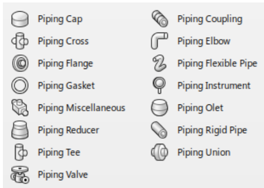
Figure 2. Types of piping parts in CATIA
